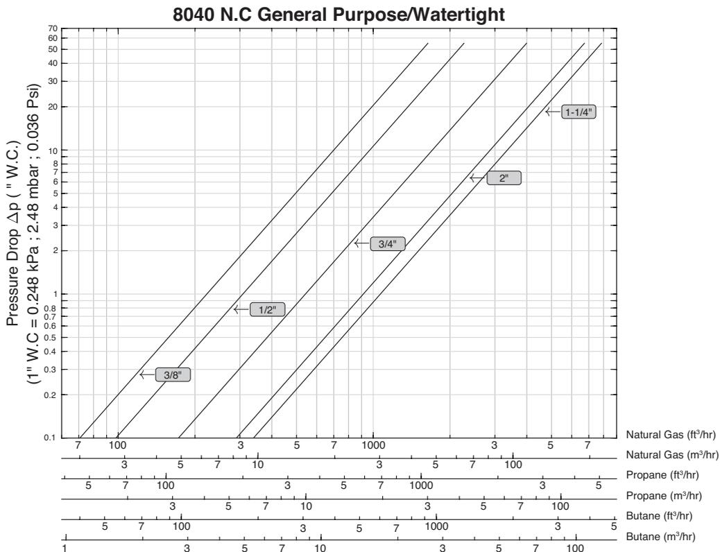
**Note:** Flow curves are based on the following standard conditions: 5 psi (0.3 bar) inlet pressure and 68°F (20°C) fluid temperature.
