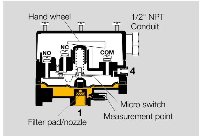
Pressure switches which lock off after switching can only be unlocked with a manual reset, see page 16 (Resetting pressure switches with manual reset).
