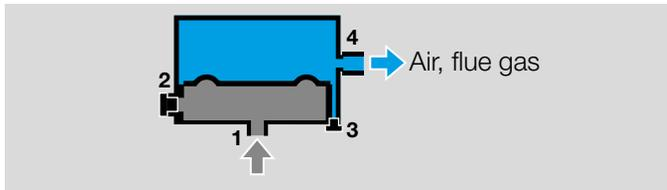
The negative pressure is measured in the upper diaphragm chamber, port **4** (or **3**). The lower diaphragm chamber is ventilated via port **1** (or **2**).
