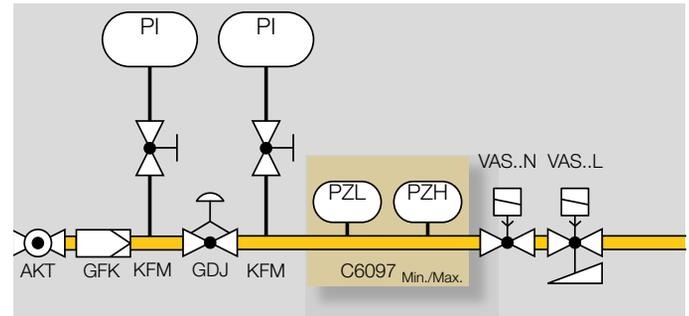
If the pressure is either too low or too high, the min./max. pressure switch (PZL/PZH) switches in order to avoid start-up or to initiate a safety shut-down.
