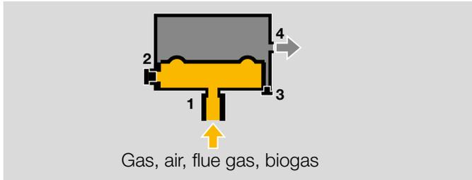
The positive pressure is measured in the lower diaphragm chamber, port **1** (or **2**). The upper diaphragm chamber is ventilated via port **4** (or **3**).
