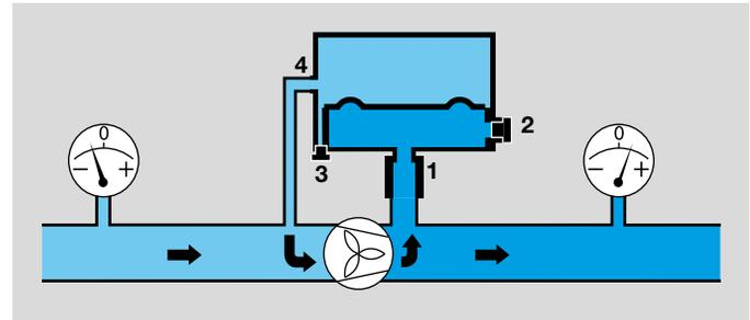
The higher absolute pressure is connected to port **1** (or **2**), and the lower absolute pressure to port **4** (or **3**). The remaining ports must be tightly plugged.
