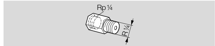
In the case of high pressure fluctuations, we recommend using a restrictor orifice (contains non-ferrous metals):
