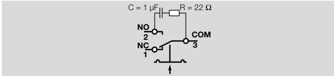
In the case of high humidity or aggressive gas components ( $H_2S$ ), we recommend using a pressure switch with gold contact due to its higher resistance to corrosion. Closed-circuit current monitoring is recommended under difficult operating conditions.
