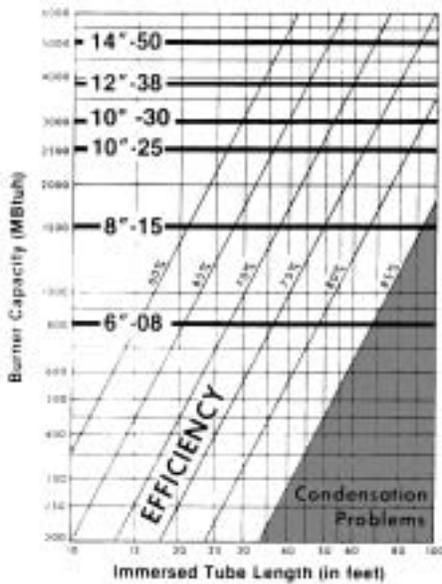
Many factors affect overall system efficiency. Tube length is the most important. The graph above shows approximate tube length required to attain a given efficiency. Typical installations run in the 70% – 75% range. Space considerations (including tube displacement) may limit possible tube lengths and so reduce efficiency. Above 85% efficiency, there is a risk of condensation-caused tube damage.
