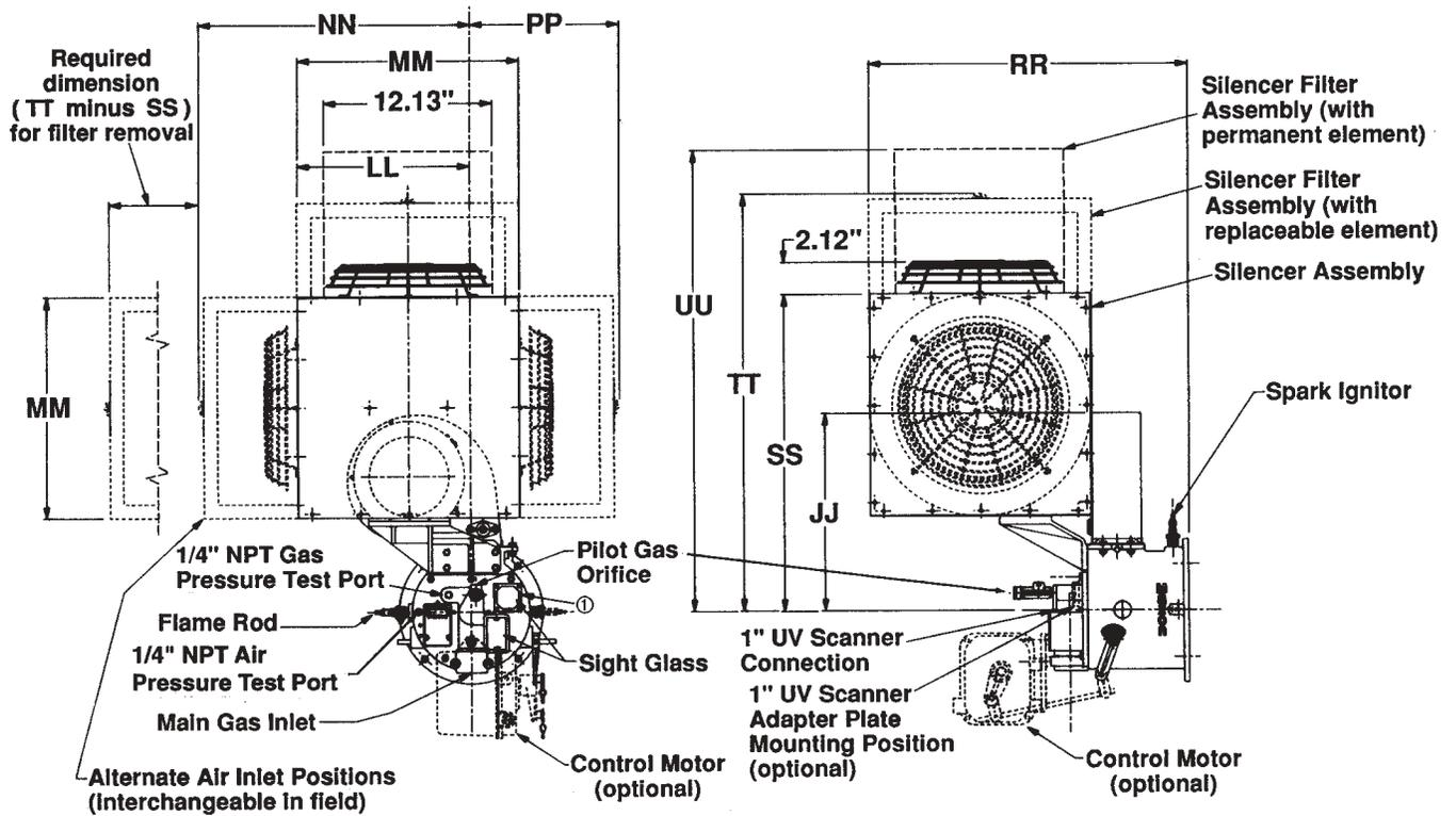
① NOTE: Upper sight glass replaced by UV Scanner Adapter Plate, 1" NPT, if used (optional)
