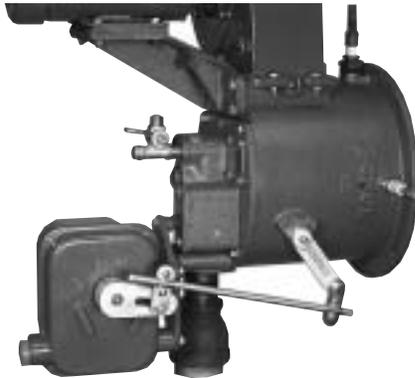
**Automatic burner with Maxon hi/lo control motor**
