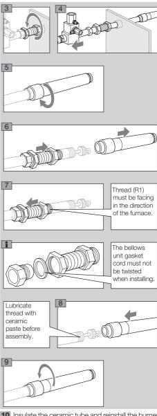
10 Insulate the ceramic tube and reinstall the burner, see page 3 (Installation).
