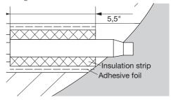
3 Check that the burner block hole is not blocked, e.g. using a wooden stick.
