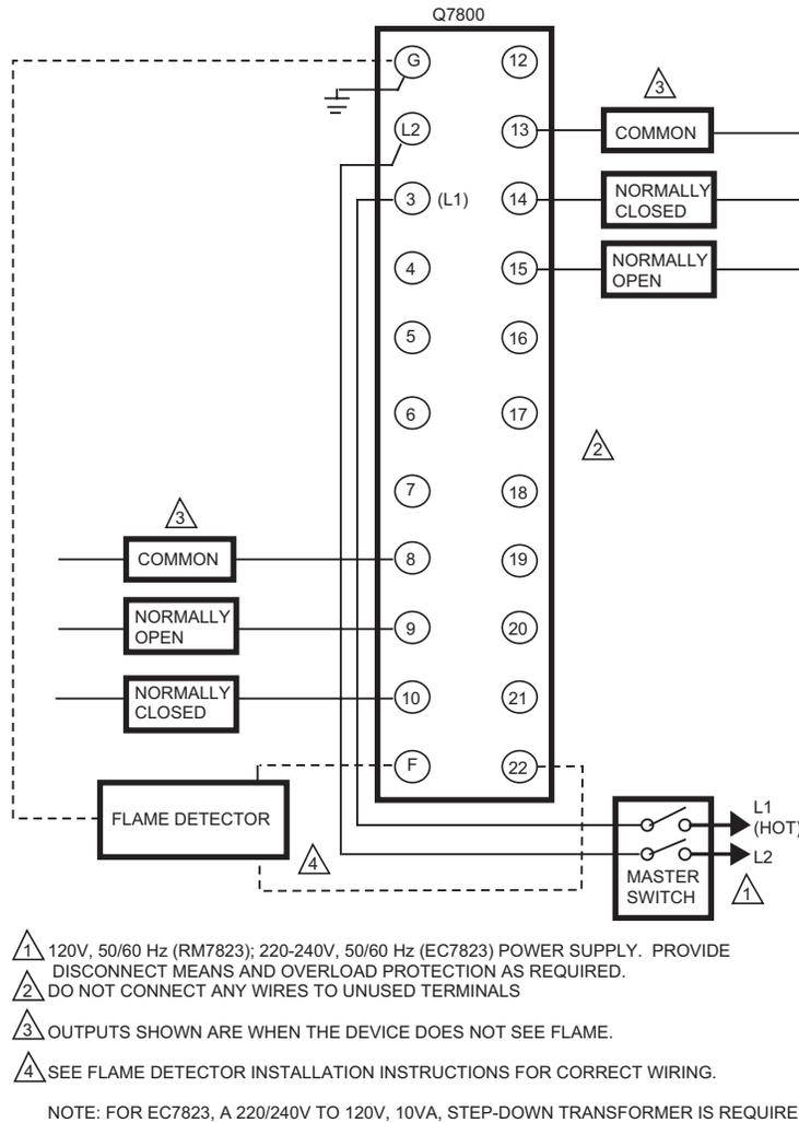
**Fig. 2. Wiring subbase for EC/RM7823A.**
