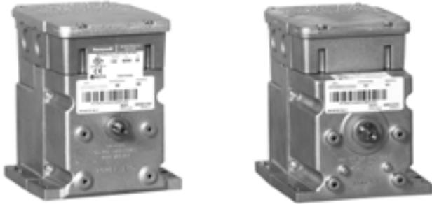
**Series 62 Modutrol IV™ Motors Spring Return and Non-Spring Return floating control motors used with controllers that provide a switched spdt or floating output to operate dampers or valves.**
